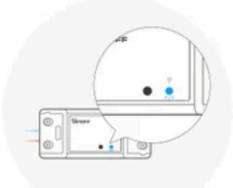
Check Wi-Fi LED indicator flashing status (Two short and one long)
