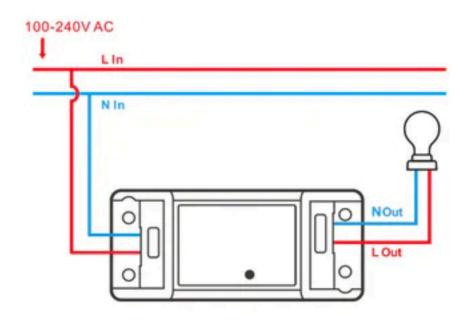
\*Please power off before wiring. To avoid electric shock hazards, do not operate any connection or contact the terminal connector while the device is powered on!
