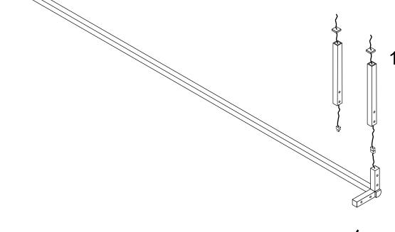
1. Thread the power cable though the foot and connect it to the plug on the joint.
